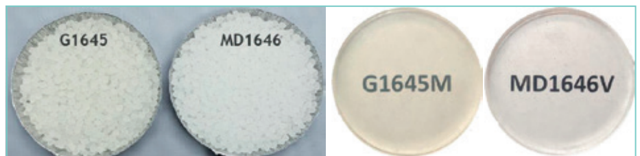
Fig. 4: Visual comparison of Kraton G1645 and Kraton MD1646 pellets (left) and solution cast film (right)
