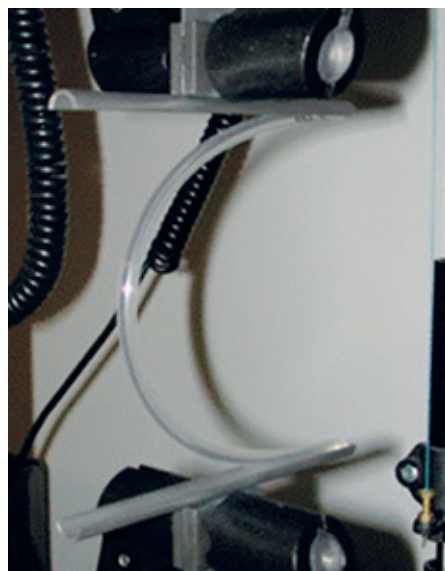
Fig. 1: Photo of test set-up developed to measure kink resistance of tubes
